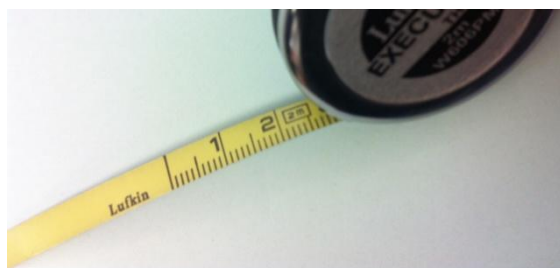
Figure 1b. Metal tape showing blank space before the zero mark
