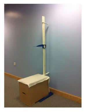
Figure 2. Assembled stadiometer mark (first 3 segments) with positioned anthropometric box.
