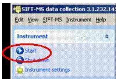
10. A script box will open on screen indicating the progress of the start-up. It will report the voltage ramp on the source and the attempt to strike the source discharge. This is not always successful. If successful, a pink glow from the source can be seen through the grill at the top of the left side panel of the SIFT/FA-MS. In the read-backs, pico A will start to rise.
