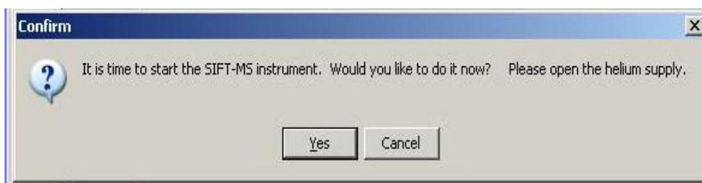
9. a) If the instrument is installed in SCBR Consulting Room 16 the helium supply is turned on and off using the hand wheel on the top of the cylinder and not the black knob on the regulator valve. The wheel is turned anti-clockwise to open.
